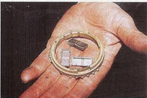
Ultimately this is what happens within a Type-9 when gearchanges are consistently rushed, the baulk rings shatter and the hub plates/inserts are also wrecked. A complete overhaul is then required.
