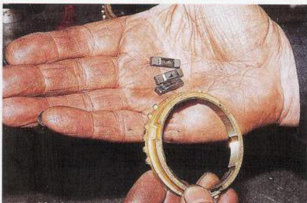
These are new baulk ring and three intact hub plates (inserts). All the tabs are in good condition and the working surfaces are clean and shiny. These are genuine Ford components.
