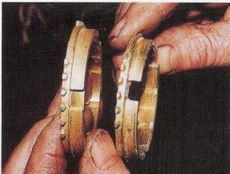
A sign of trouble is breakage of the edges of the hub plates (inserts). The sheared edges can dig into the baulk ring, so that the insert cannot slide out of engagement as designed. It can then be difficult/impossible to take the car out of gear.
