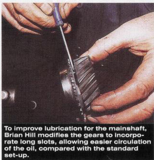
One of Brian's effective mods made is to upgrade the standard 1.6/1.8/2-litre gearbox to incorporate a long (high) ratio first gear. The original cog is removed from the laygear, and splined to accept a new, higher ratio.
