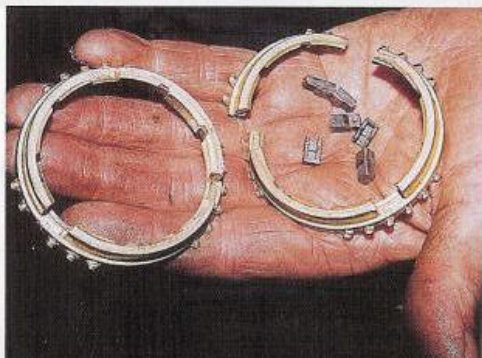
Another problem to watch out for is the breaking away of the tabs within the baulk rings, this is the first stage of the ring breaking up. Shown here are a new baulk ring (on the left) and one with a tab missing (on the right).
